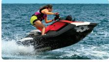
Extended Range VTS<sup>™</sup> (Variable Trim System) Offers double the range of the regular VTS<sup>™</sup> for greater ease when executing tricks.
