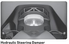
3 steering positions to quickly control the stifness. It adds riding precision by removing undesired input in rougher conditions. It provides a premium feeling and improved control to the rider.
