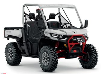
82 hp / 69 lb-ft, Rotax® 976 cc, V-twin, liquid cooled
